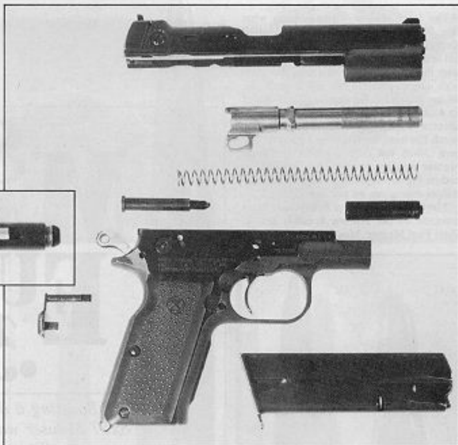
The Bren Ten uses the time-proven Browning short recoil system and is easily broken down for routine cleaning, maintenance, or repairs.
