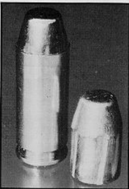
The fired 10mm bullet penetrated 9 inches of wood without distorting. Shown with .45 slug and 10mm load.
