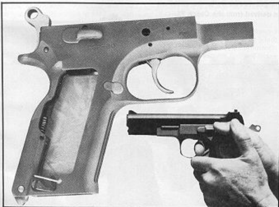
At the head of the frame, a two-stage detent offers the option of full or partial ejection of the magazine. The pistol is slightly smaller than the 1911 Al Colt, with identical trigger reach when cocked.
