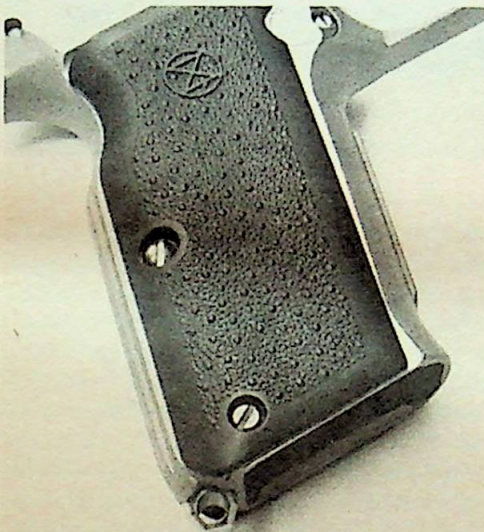
The small screw head at the bottom of the grip is a selective magazine catch. It may be set to eject the magazine fully, or hold it partially ejected for manual extraction. Extension of the mainspring retainer serves as a lanyard ring.
