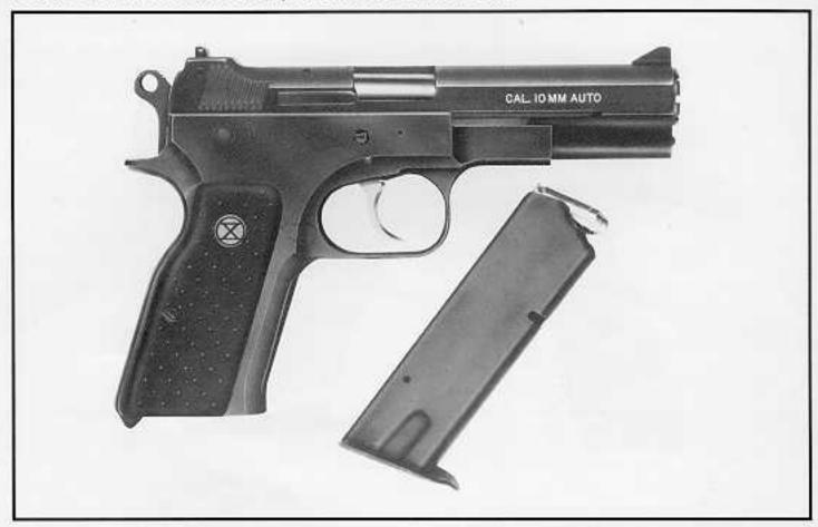
The Bren Ten Military/Police Model is a full-size, heavy-duty, semi-automatic, defensive combat service pistol designed to fire the 10mm Auto pistol cartridge. It is identical to the Standard Model except the finish is completely matte and all black.
